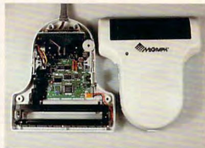
Inside Migraph's Scanner: The scanning window and light source are at the bottom, and imaging optics are at the top.
