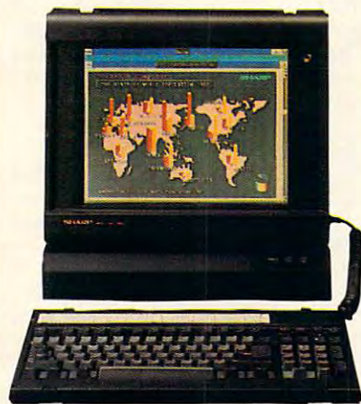
Sharp's portable Multi-Color 386 features a color-LCD VGA screen.
