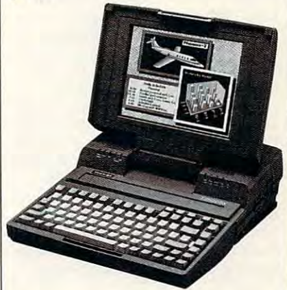
The T3100SX is Toshiba's first battery-operated 386SX portable.
