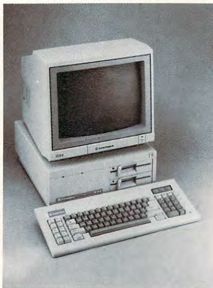
The Commodore PC10-III is an XT-compatible computer designed for educational and small-business use.
