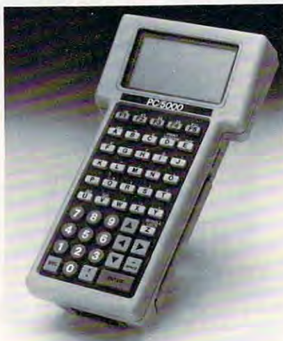
The hand-held PC/5000 uses the MS-DOS operating system.
