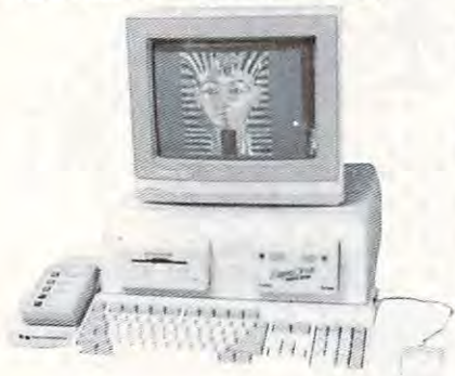
The Amiga 500 Command Center places disk drives above and behind the keyboard.
