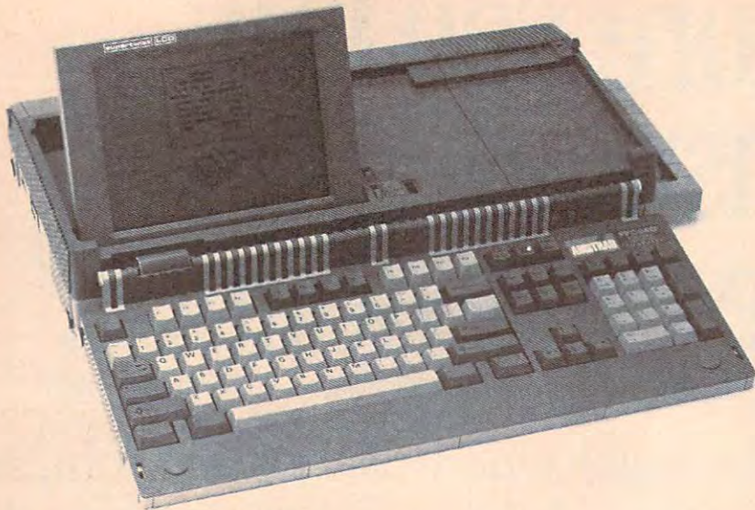
The Amstrad PPC 640 has its own built-in modem.
