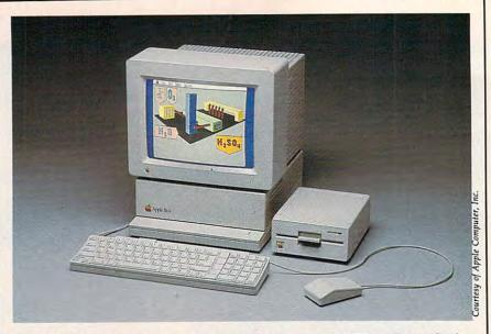
The Apple IIGs computer, shown here with the AppleColor RGB monitor and 5¼-inch drive, features 256K of RAM, high-resolution graphics, high-quality sound synthesis capabilities, and complete compatibility with existing Apple II software.
