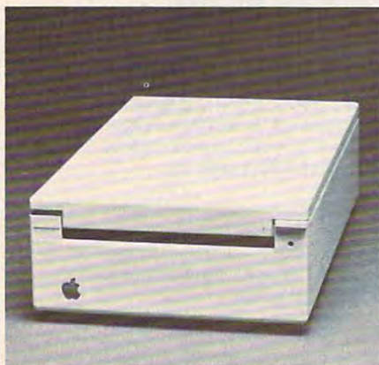
Apple Computer's UniDisk 3.5 is a double-sided floppy disk drive that stores 800K of data, one of a growing number of 3½-inch drives for popular microcomputers.
