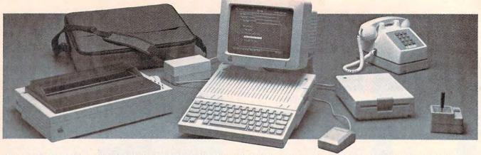
The Apple IIc, with optional 9-inch monitor, Scribe thermal transfer printer, AppleMouse II, external disk drive, joystick, modem, and carrying case.
