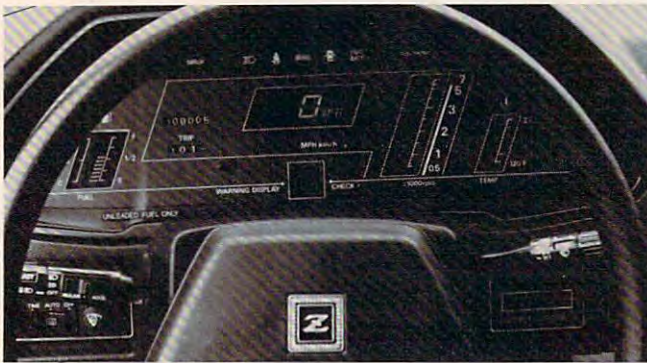
The digital instrument display of this 1983 Datsun 280ZX illustrates the numerous features now controlled by microprocessors in cars.
