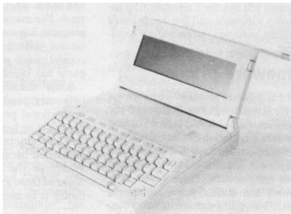
*The Commodore LCD Personal Computer can run on 4 AA alkaline batteries for 15 hours.*
